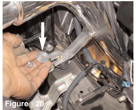
Figure 17 Lower the intake into the engine compartment and into the bumper area.
