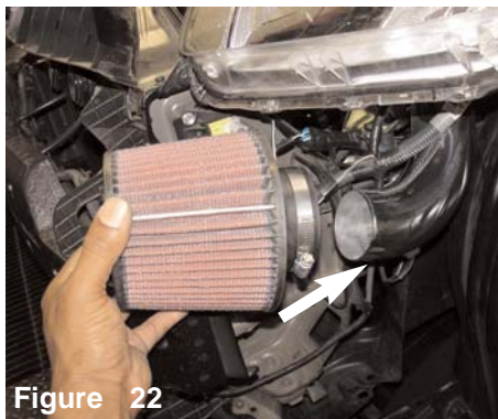
Figure 19 The intake bracket is aligned to the vibra-mount stud while the other end is inserted into the throttle body hose.
